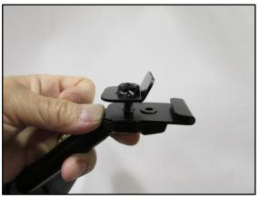
2. Place upper and lower mounting brackets on mirror arm as shown. Install 8mm bolt but do not tighten yet.
