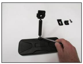
1. Thread mounting arm into mirror and tighten with 8mm wrench.
