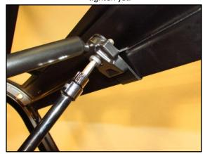
4. Tighten bolt using 6mm allen wrench.
